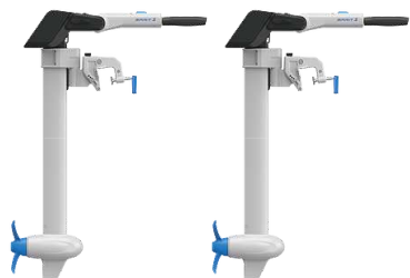
2 x SPIRIT 2 Longshaft (Motor only) Total Power: 4 kW
