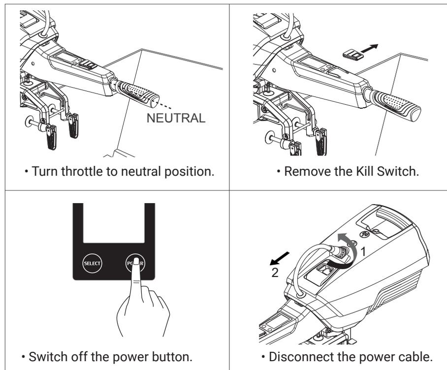
In normal operating procedure, it's recommended to stop the outboard as following steps.
