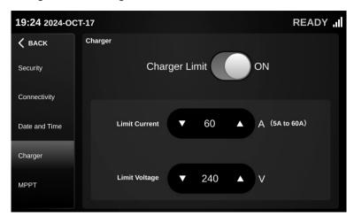
Press Input to set the maximum charging current and voltage.
